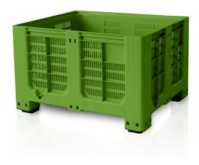
Plastic bigboxes are intended for transport, handling and storage of packed and loose goods. Their dimensions allow for maximum space usage. Stackability and easy handling are great advantages. They are crash and weather resistant. The bottom and walls have ventilation slits for air circulation. Bigboxes and be closed with a lid and stacked. 4 feet .
