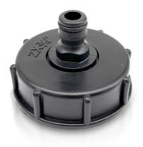
IBC reducer (adapter) DN50 Inlet - internal thread S60x6 (coarse) x external thread BSP 3/4" (fine) Outlet - quick coupling for hose with 3/4" fitting
