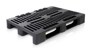
The ESD pallets out of electrically conductive plastic were especially designed for transporting sensitive electronic devices. They reliably prevent electrostatic charge and divert already existing charges. Special volume resistivity/surface resistivity: 10<sup>4</sup>< 10<sup>10</sup> Ohm. Pallets are used, without rims.
